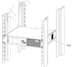
• Elevated Operating Ambient - If installed in a closed or multi-unit rack assembly, the operating ambient temperature of the rack environment may be greater than room ambient. Therefore, consideration should be
